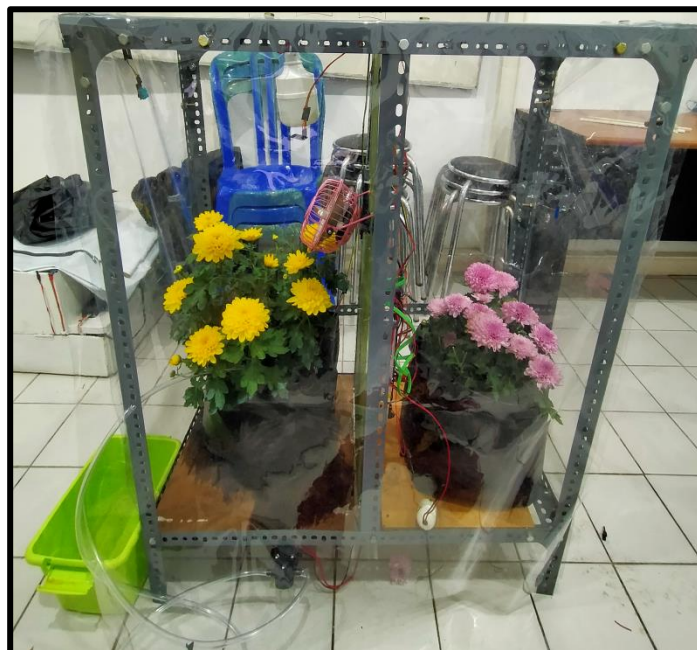
Gambar 9. Alat monitoring bunga Krisan
