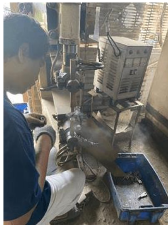
Gambar 7 Proses Mesin Spot Welding
